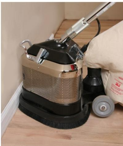
The three-head sanding design will sand the entire floor, including edges and wall lines.
