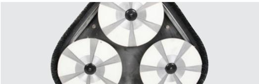
Three cast aluminum drive plates that have six pie shaped hook faces attached.
