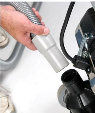
A vacuum-ready dust pipe design easily fits a 1.5 inch vacuum hose for use with a dust control vacuum system.
