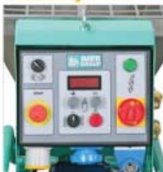
An onboard computer balances the spray rate with the pumping volume, this prevents clogging.
