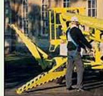
Fully proportional hydraulic outriggers make setting up and leveling quick and easy even on gradients.
