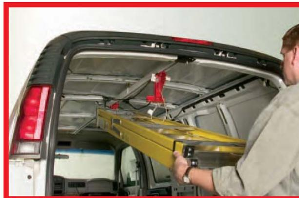
**1. Place the top of the ladder into the front cradle assembly.**
