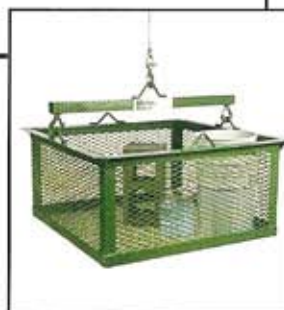
BASKET (with spreader bar) 800 lb. capacity 36 3 / 4 L x 36 3 / 4 W x 18 1 / 2 H 400 lb. capacity 30 3 / 4 L x 20 3 / 4 W x 12 1 / 4 H
