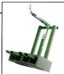
BLOCK FORK 800 lb. capacity 24 1 / 2 L x 24 1 / 2 W x 34 1 / 2 H For lifting 8 x 8 x 16 block
