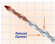
Spira-Lok™ Asymmetrical Ties are dual diameter Spira-Lok™ Stainless Steel Helical Wall Ties designed for use in connecting soft veneer materials to a hard back-up. Typically a larger installation pilot hole is required in hard substrates, such as concrete or brick, than, for example, in a soft veneer mortar.
