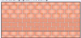
For lintel replacement, the area to be supported is defined by drawing lines at 45° from the corner points of each side of the opening.
