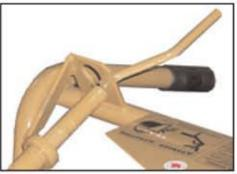
Cutting depth is controlled easily though the depth control lever located at the operators right hand side. With a heavy duty sealed bearing in place the lever is easy to control and the tight threads located at the front near the wheel allow a wide range of cutting depths. With the blade on the opposite side from the depth control threads dirt buildup is prevented and because the threads are closed to one end at all time shaft bending is prevented.
